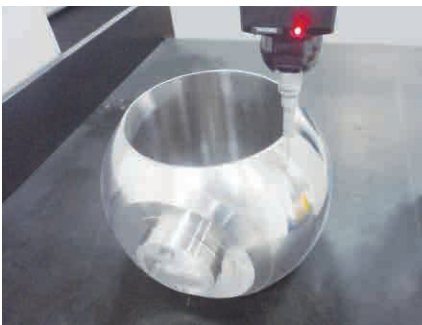
Roundness inspection by CMM (Coordinate Measuring Machine)
