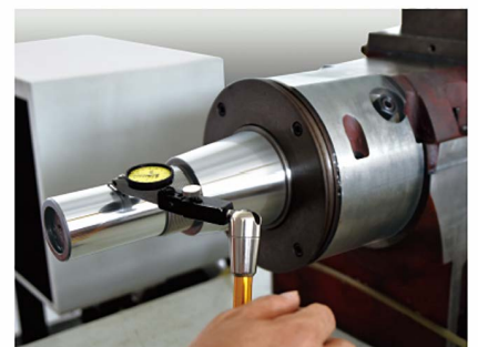
The spindle rotation runout accuracy test
