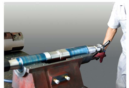
Precision assembly of spindle and alloy bearing to obtain the best accuracy
